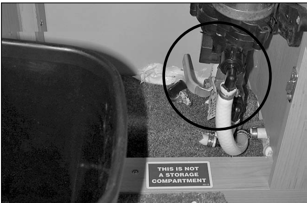
Picture G-P1: Selector valve position for supply from the interior fresh water tank.
